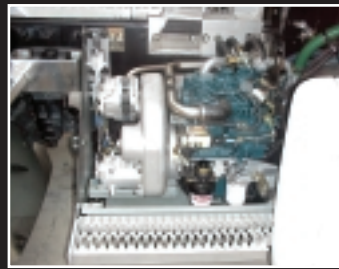
The Willis Auxiliary Power System provides all the power requirements for a typical Class 8 truck, except pulling the load.
