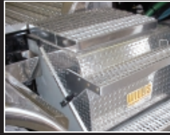
The Willis APU is lightweight and fits comfortably on the frame rail.
